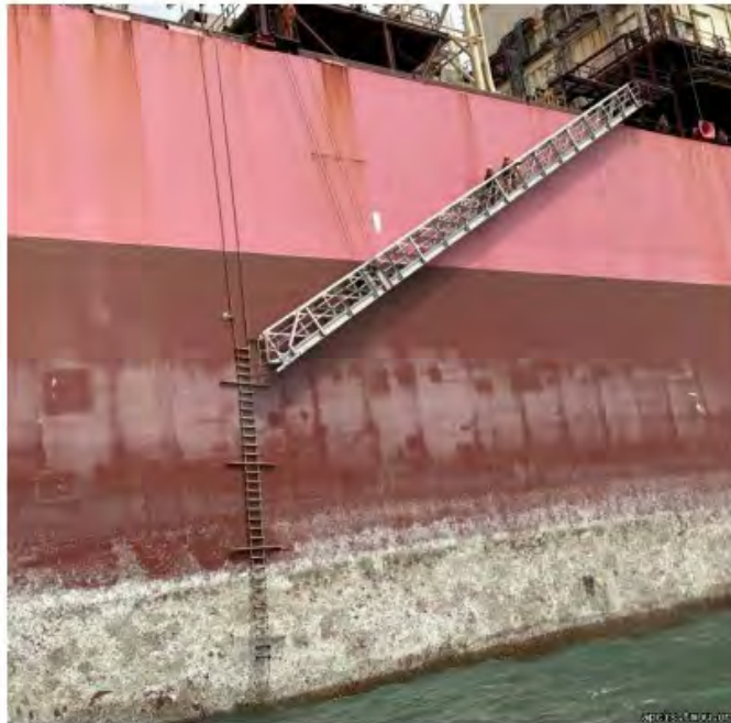
Photo 2: Example of non-compliant combination pilot ladder arrangements.
