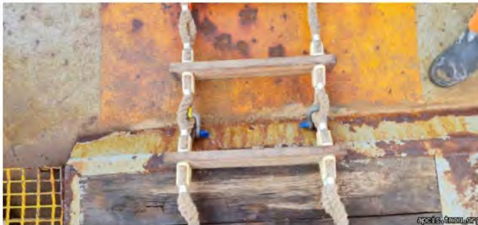
Photo 5: Unsafe pilot ladder securing arrangements.
