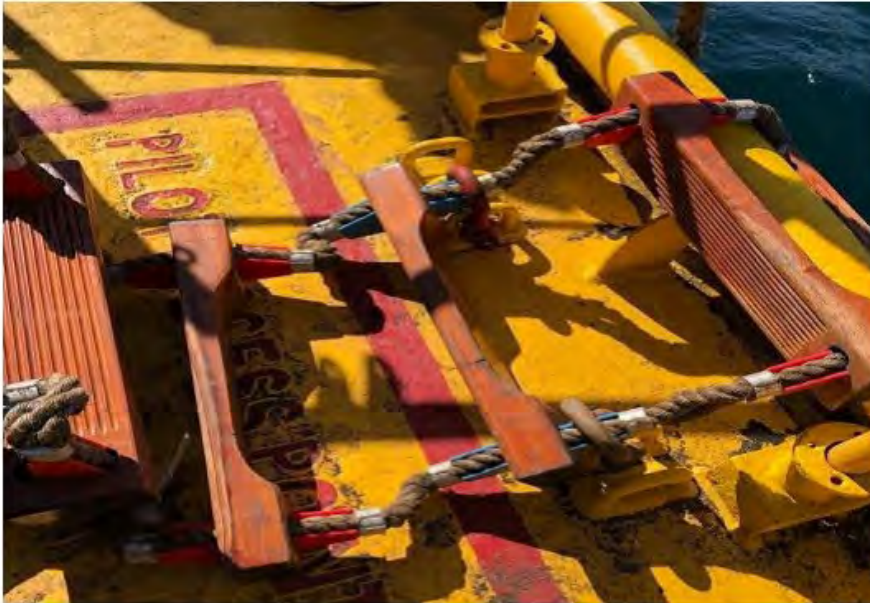
Photo 4: Unsafe pilot ladder securing arrangements (Reproduced with permission from Fremantle Ports).
