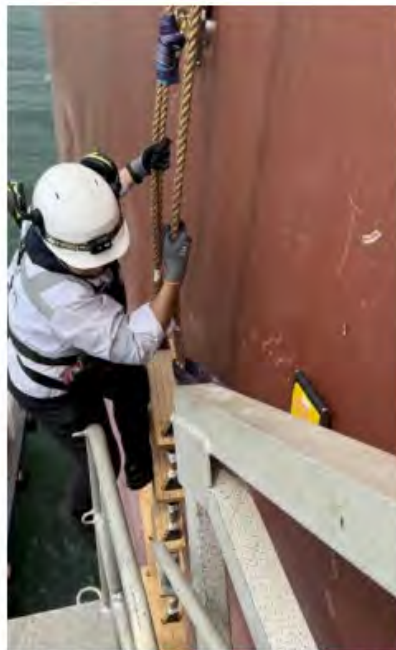
Photo 3: Person unable to safely access accommodation ladder platform from pilot ladder.
