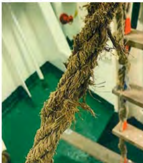
Photo 10: Frayed side rope.
